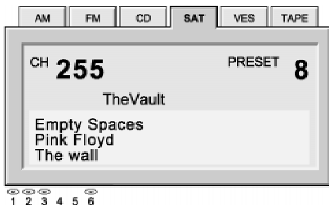
Figure 14: VES display in SAT mode. Channel Name, Song, Artist, and Album information is displayed by VES.
