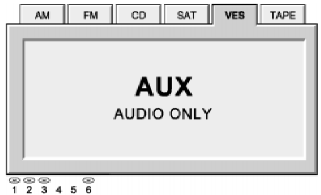
Figure 6: Display for Audio only device, such as MP3 player connected to VES AUX port.
